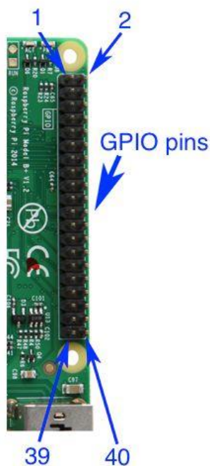
Raspberry Pi B Rev 2 P1 GPIO Header
